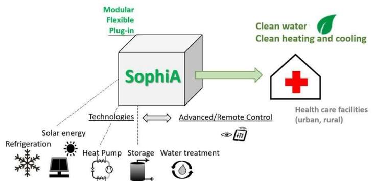
Figure 1.2: Innovative, modular, flexible, affordable and efficient solar powered SophiA system combining PV panels mounted on top of containers with multi-temperature refrigeration system, battery and controls, ice thermal energy storage, water purification and treatment, hot and cold water storage.
