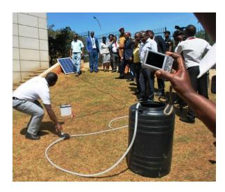
The Department of Agricultural and Biosystems engineering in partnership with Perdue University in Indiana USA developed a solar-powered Irrigation pump as a cheap and reliable solution for small scale farmers that form the bulk of farmers in the world. The entire system can be assembled at a cost of shs. 6.5million.
